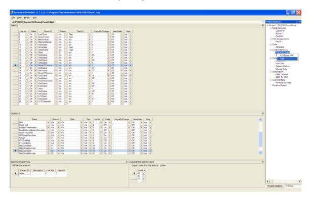
To set up the I/O to signal a Tool Comp Source to do a Reset Trend on all its Compers, use the input line specified in the Source's Reset# field (see 2.3.1.10) and specify the ResetTCSource event. Note the highlighted Input row in the above screen shot. Line 14 On sends the ResetTCSource event to whatever Tool Comp Source has its Reset# set to 14. Note that inputs 15 and 16 are being used for the other two Sources.
