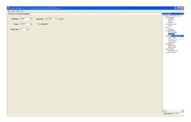
The Ovation Tool Comp hardware uses RS485 to receive command strings from the U1000. Specify the COM port used for the 485 connection to EZComp devices and the baud rate being used by the devices (the default is 9600). The N, 8, 1 indicates parity = none, data bits = 8, and stop bits = 1.
