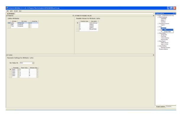
Note the Set Using column for the Lathe attribute in the above screen shot. It uses an InParameter to select the value. An InParameter is a binary number formed using one or more input lines (see 2.1.2). When the Lathe row is selected in the attribute grid above, the "Set Using" definition for the attribute is shown in the lower part of the screen.
